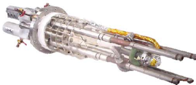
R&D and manufacturing of 600A HTc current leads prototype for CERN. In order to reduce the heat load into the superfluid helium, D.C. current leads based on high temperature superconductors have been designed.
