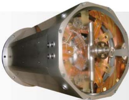
Near IR camera designed for ground based application. Installed in Granada Observatory. Compact and light weight, is cryogenically cooled to work in temperature (77K) by an half-filled anular tank inside the vacuum dewar.
