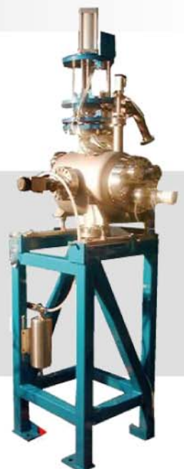
Safety shutter placed in the transfer line. In the closed position it stops the electron beam. SOLEIL Synchrotron.
